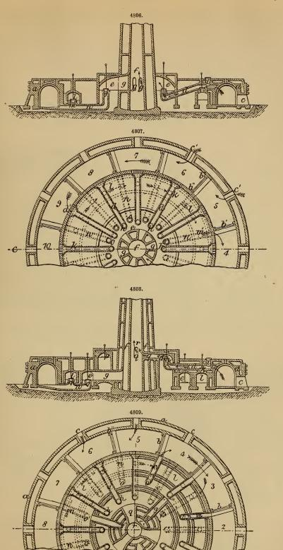
the doors or dampers made up in several parts, each small enough to be introduced through the entrance c; by this means the doors  $b, b^2$ , may be inserted or removed by hand through the same apertures by which the kiln is filled and emptied.
